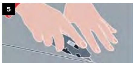
**6.** Using the trimmed edge of the first length as a guide, cut the edge and remove the surplus.
