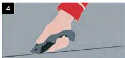
**5.** Position the second length of carpet, with the edge of the first length overlapping the second by approximately 50mm.
