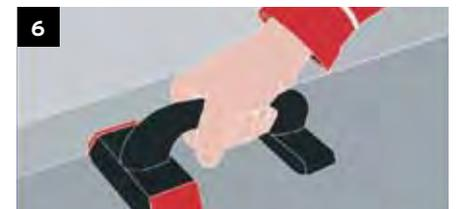
**6.** Using an Araseur or a sharp knife, trim the carpet to fit against the perimeter walls.
