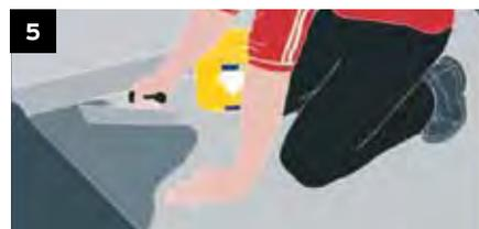
**5.** Fold the sheet half way back taking care not to disturb the positioning of the flooring. Apply the recommended adhesive onto the subfloor using the application techniques previously described, from 20cm inside the first guide line to 20cm inside the next.
