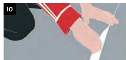
**10.** Immediately relay the second piece starting at the centre, press the edge into the seaming adhesive along the entire length. Any fullness of carpet should be dissipated away from the seam.
