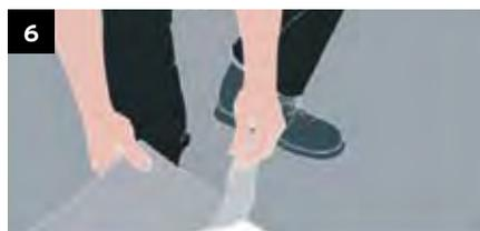
**7.** Prepare a compression seam joint by overlapping the edge of the first piece with the second piece by approximately 3mm.
