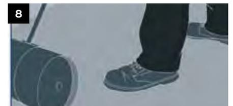
**8.** When the floor has been completely covered re-roll the area again to maintain good adhesive contact.
